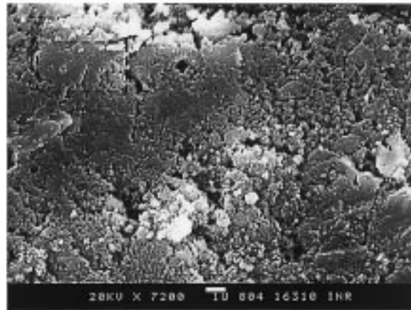
Fig. 4. SEM micrograph of an MPC sample (pressure 1.8 GPa, density 68% TMD). Box indicates a clearly densified area.
